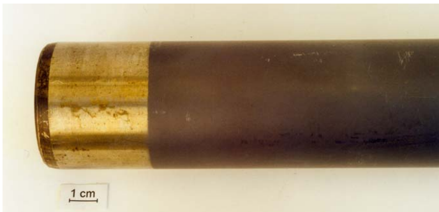
Figure 4 : Unstressed pin (D6) with Te'Strake 7409 heat curing solid bonded film
