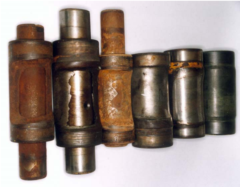
Figure 2 : Typical wear patterns observed in the field
