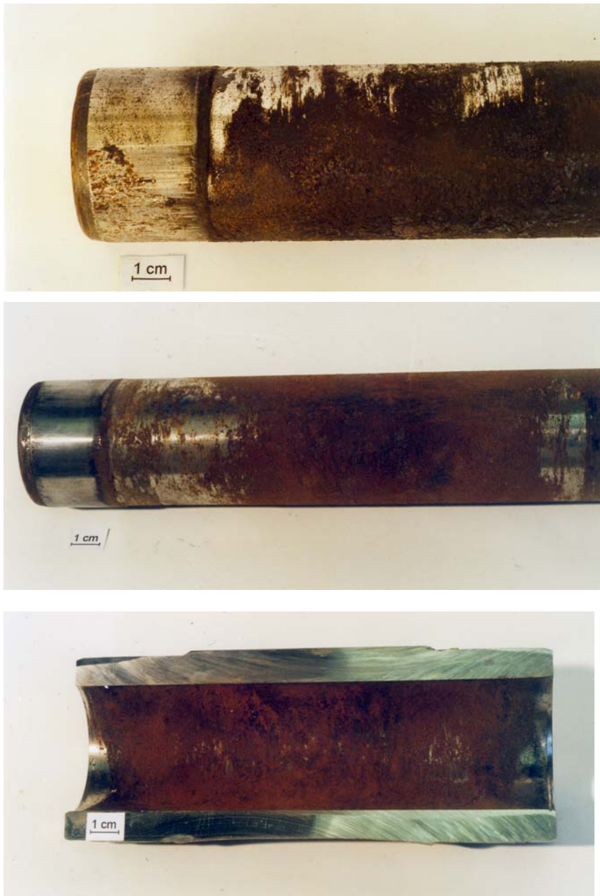
Figure 5 : Solid bonded film pin after 280 operating hours in an unsealed chain section (top). Pin after 1,000 operating hours in an unsealed chain section (centre). Inside of bush after 1,000 operating hours (bottom).
