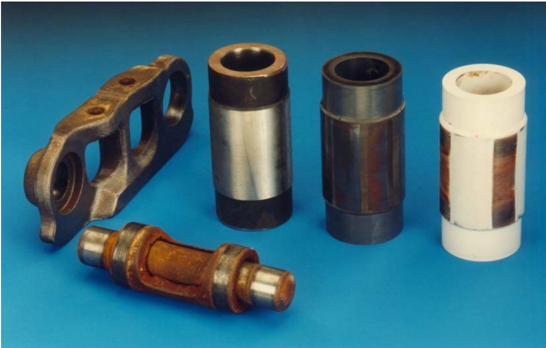
Figure 1 : D6D-Buschings in steel and monolithic ceramics having typical wear patterns and a worn D4D-Bushing
